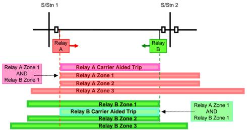
Where the signalling equipment has an output which indicates that the signalling channel is out of service, this can be connected to a Status Input called *Carrier Recv Guard*. On energisation of this status input the relay will revert to a time stepped distance scheme.
