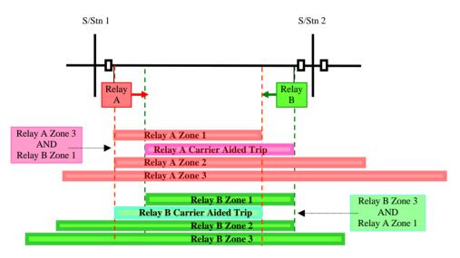
The relay is arranged to send a signal when its Zone 1 picks up.
