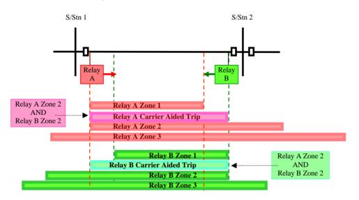
The relay is arranged to send a signal when its Zone 2 picks up.
