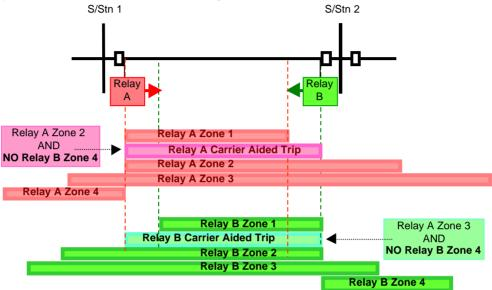
When the Zone 2 instantaneous element picks up, the relay waits for a "blocking signal" to be received. If no blocking signal is received during a set time delay (known as the Permissive Trip Time) the relay will cary out a "Carrier Aided Trip". If, during this time delay, a blocking signal is received, the Zone 2 time delay will remain in place, and the relay will carry out a Zone 2 trip after the Zone 2 Time delay.
